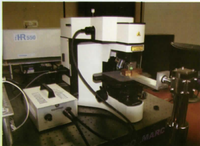
Figure 1: Fiber coupled Raman Microscope.
