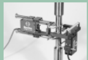
3542 axial model used simultaneously with a 3575 transverse model.
