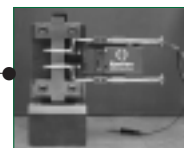
3542 with composites compression fixture for ASTM D695.
