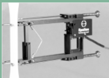
3542 with a 2" gage length and ±25% measuring range.
