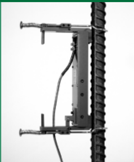
3543 with 100 mm gage length and 100 mm measuring range.
