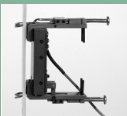
3543 with 50 mm gage length and 25 mm measuring range.
