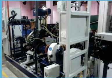
Two Cylinder Engine with Eddy Current Dynamometer
