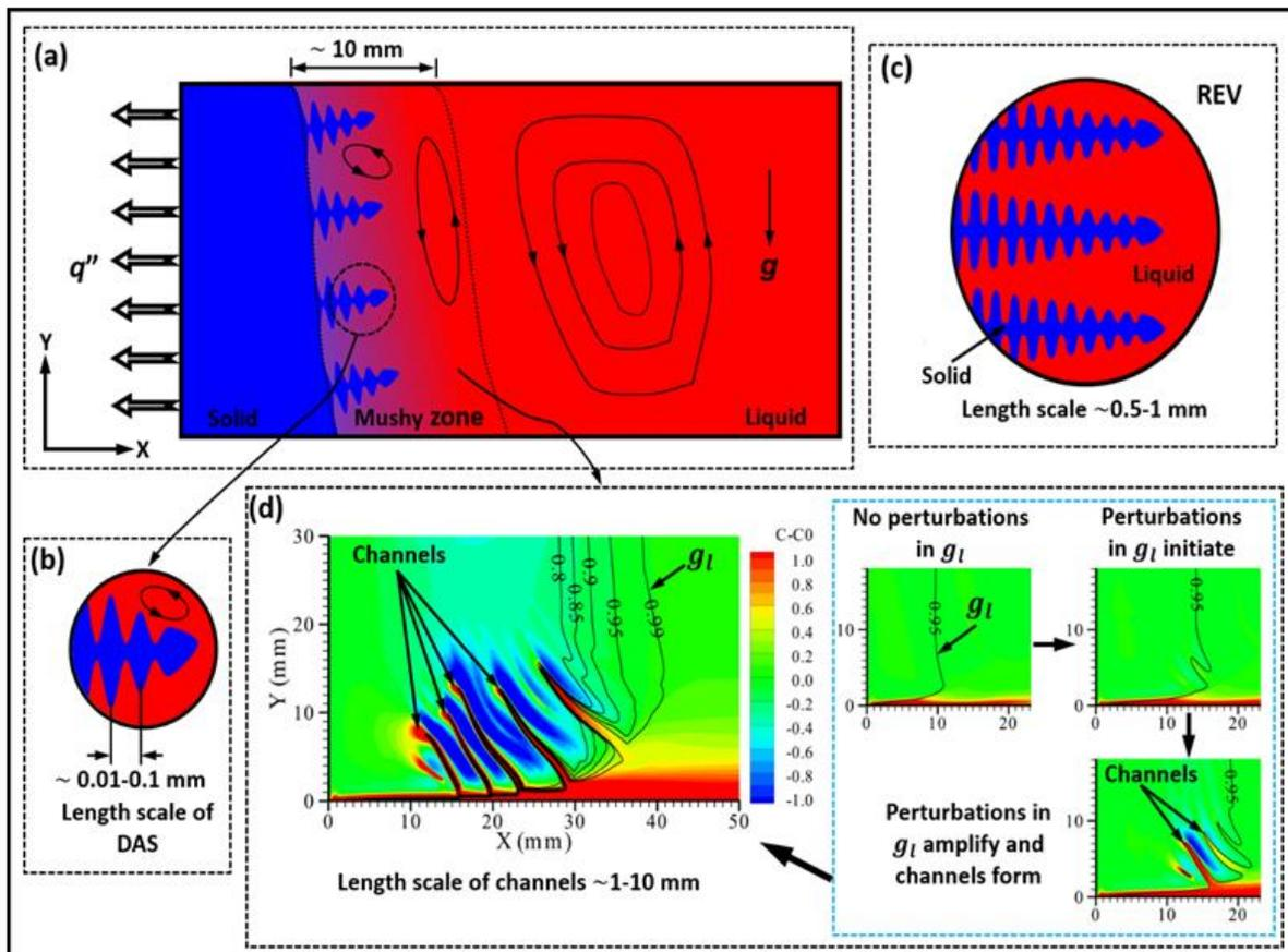
Figure 2: Illustration of the physical scales and the formation of channel segregates phenomenon during columnar solidification (a) system (macroscopic) scale, (b) grain scale, (c) representative elementary volume (REV), (d) formation of channel segregates.
