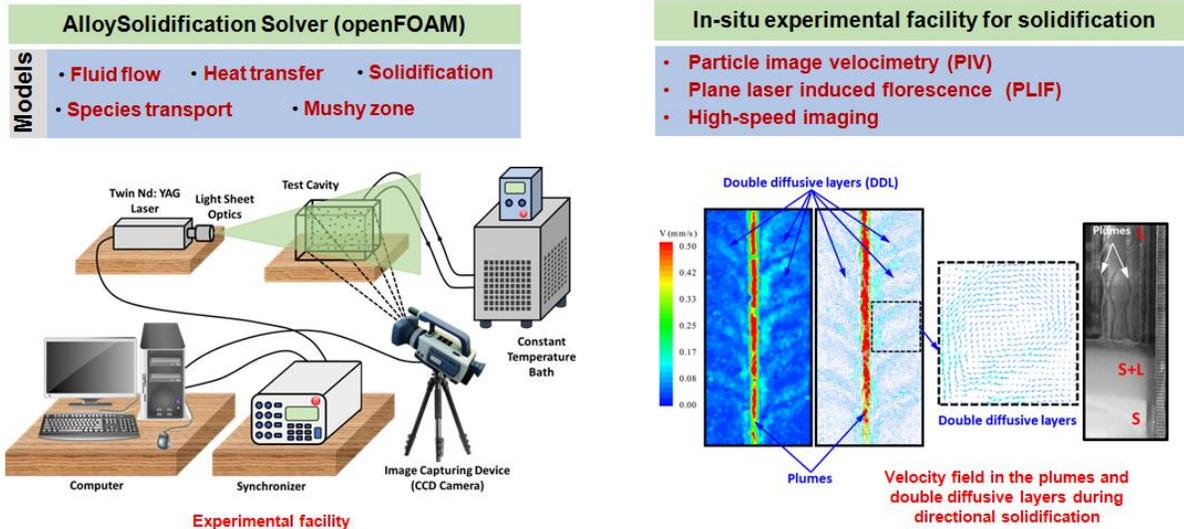
Figure 1: Opensource AlloySolidification software, and in-situ PIV, PLIF and imaging facility to investigate
