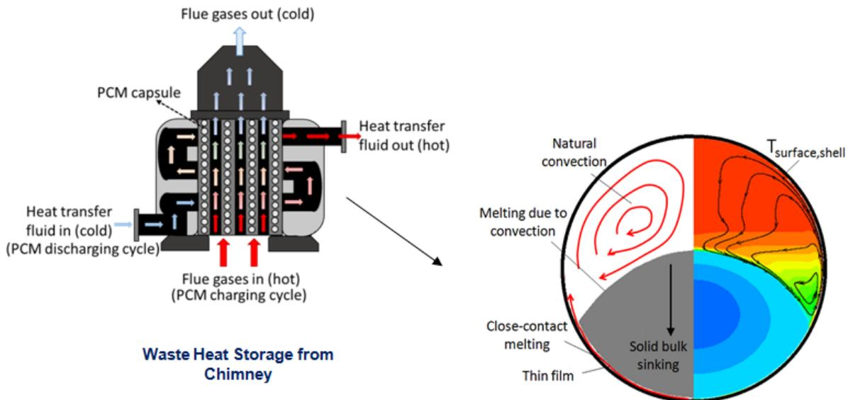
Figure 5: Fast waste heat recovery from chimney using close-contact charging of nano-enhanced phase change material composite. The physical phenomena of PCM melting during discharging in one of the spherical capsules is shown in the right image.
