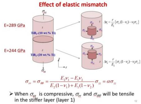
➤ Tensile stresses in the stiffer layer because of the elastic mismatch can adversely affect the compressive strength of the bi-layer composite
