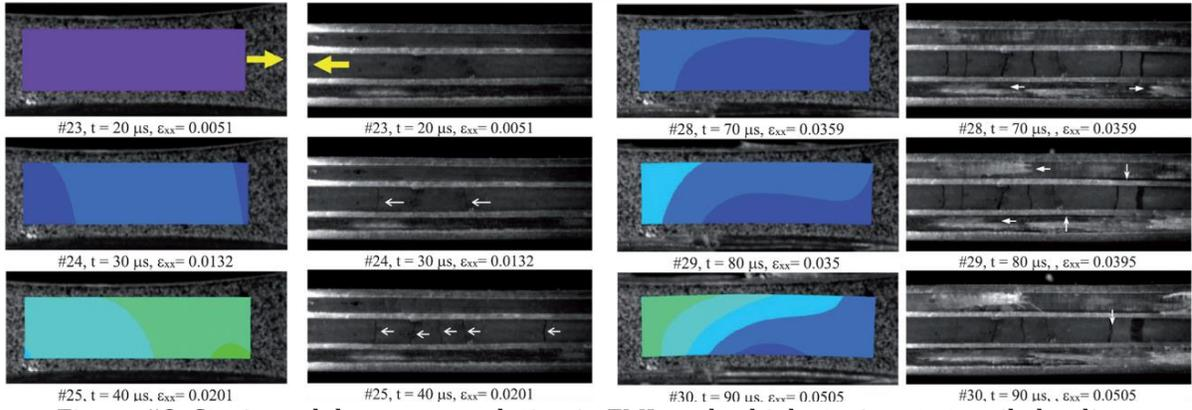
Figure #3: Strain and damage correlation in FML under high strain rate tensile loading
