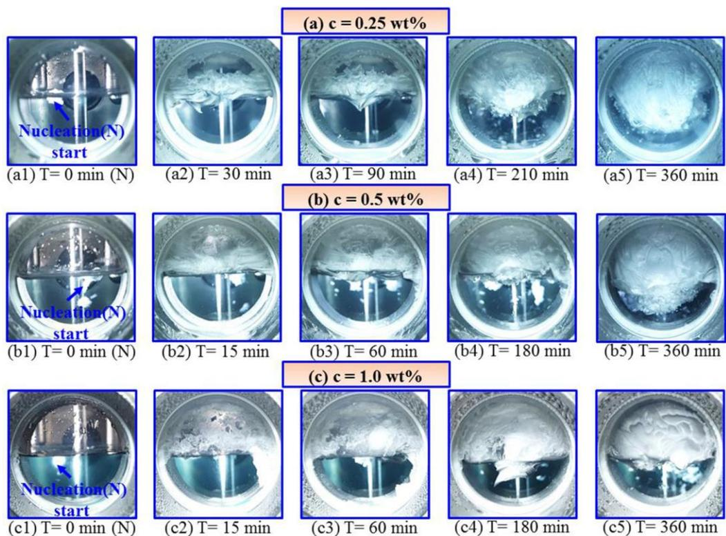
Figure #2: Visualization of CO<sub>2</sub> hydrate growth process at different Cu-Al LDH nanofluid concentrations ( $c = 0.25, 0.5, \text{ and } 1.0 \text{ wt\%}$ ) for ( $\text{Cu}^{2+}:\text{Al}^{3+}:\text{Na}^+ = 4:1:4$ ) molar ratio.
