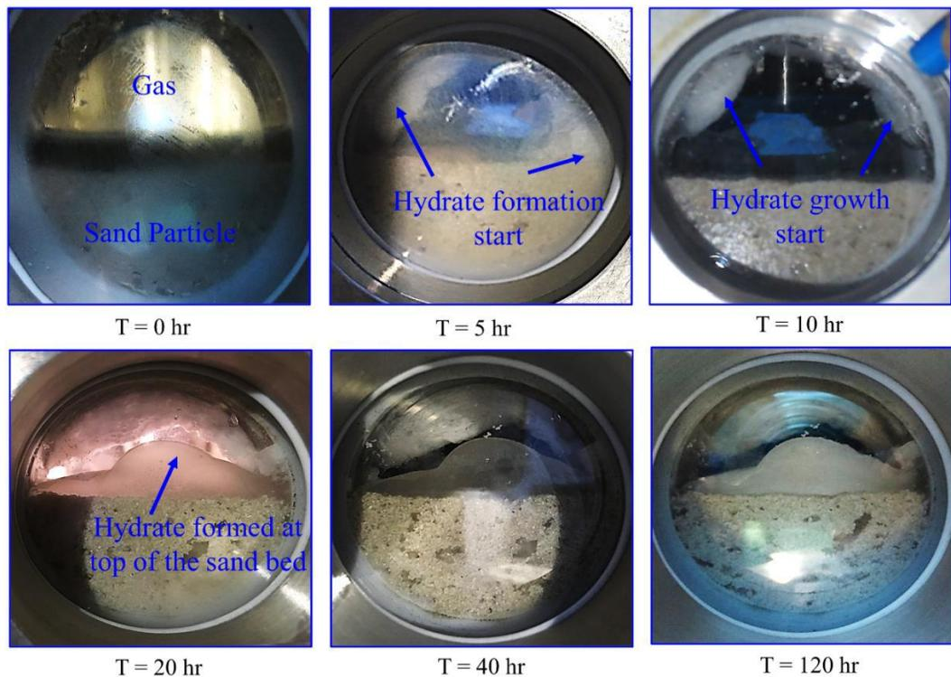
Figure #4: CO<sub>2</sub> hydrate growth visualization during the hydrate formation process
