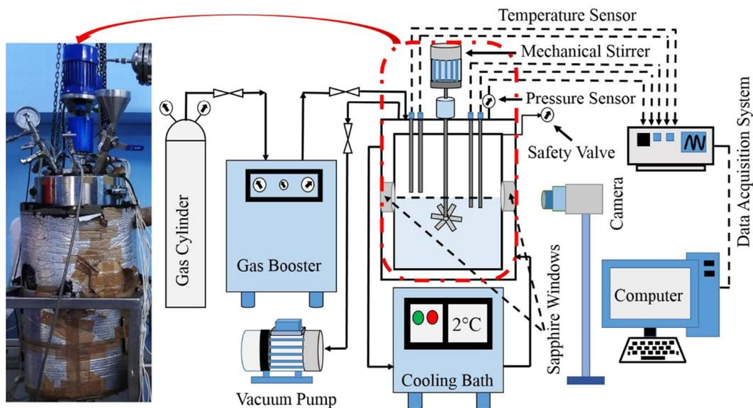
Figure #1. Schematic of the experimental setup for the study of the CO<sub>2</sub> hydrate formation process
