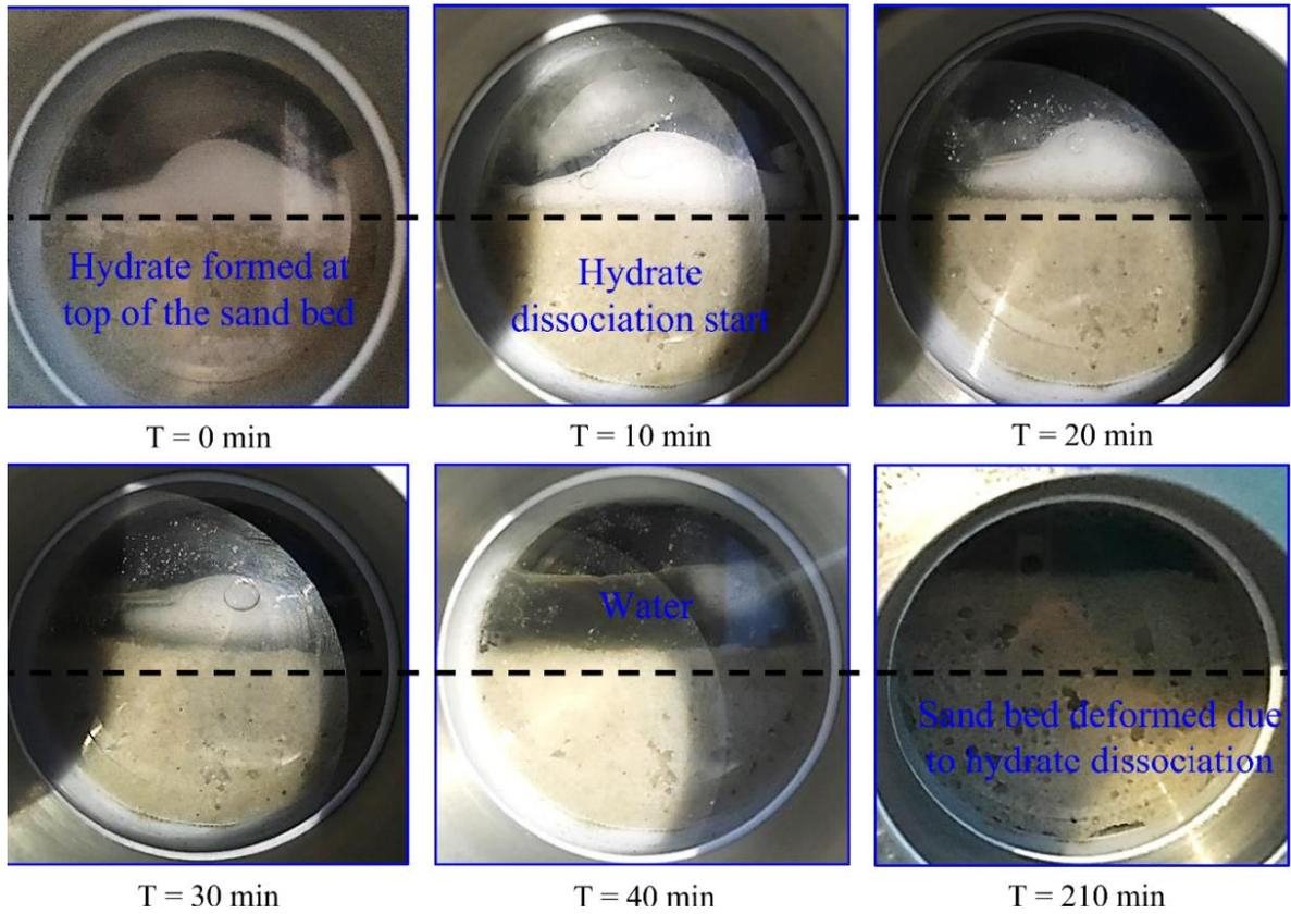
Figure #5: CO<sub>2</sub> hydrate dissociation visualization with time during the hydrate dissociation process
