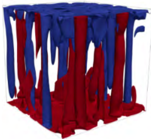
Fig: Flow organized into hot (red) and cold (blue) columnar structures
