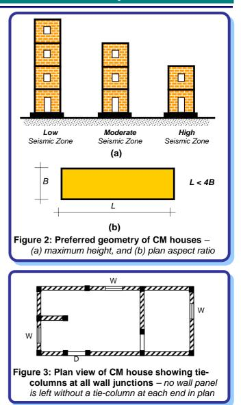
Openings in walls deteriorate earthquake performance of CM buildings. Hence, openings should ideally be kept to a minimum in number and size. Larger openings must be confined by cast-in-situ RC elements all around, otherwise a wall with large openings is considered as unconfined. Openings in all storeys must be positioned at the same location along the height of the building.
