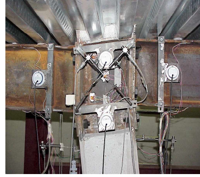
Figure 23. Column web distortion in an internal joint during monotonic test.
