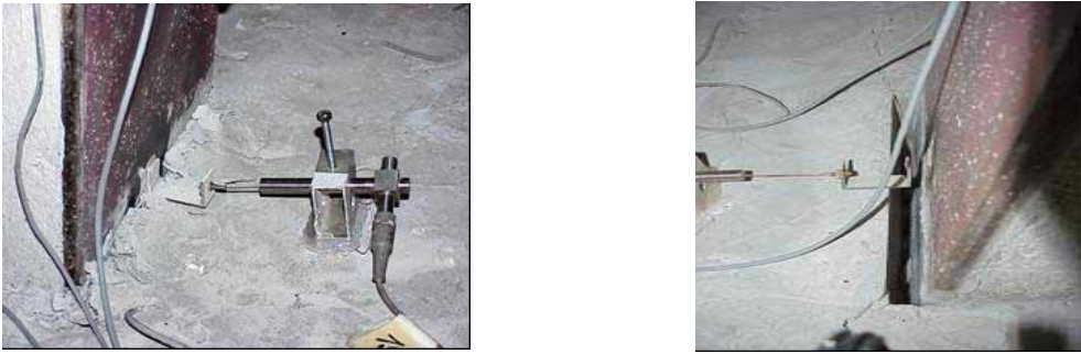
Figure 10. Monotonic test on an interior joint: a) concrete slab crushing; b) column sliding with respect to the concrete slab.
