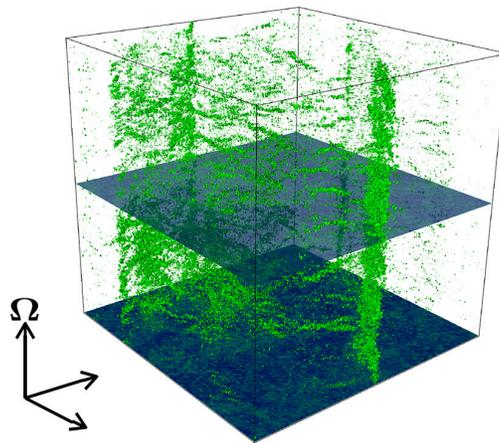
Turbulence in a rotating fluid is a common phenomenon, found in stars and reciprocating engines, amongst others. Yet despite numerous analytical, experimental and numerical experiments, its precise energy spectrum remains a topic of contention. Research from Sharma et al. has taken a fresh look at forced and decaying rotating turbulence using numerical simulations, and their results found significant differences between the two systems.
