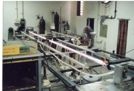
First 100 W CO2 laser fabricated at CELT
