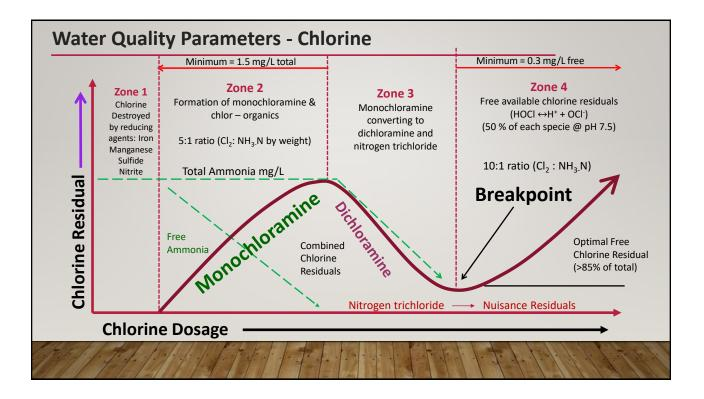
**Zone I:** Initial chlorine demand is caused by reducing agents ( $Fe^{+2}$ ,  $Mn^{+2}$ ,  $H_2S$ ,  $NO_2$ ) that consume most of the chlorine applied prior to forming combined residuals.
