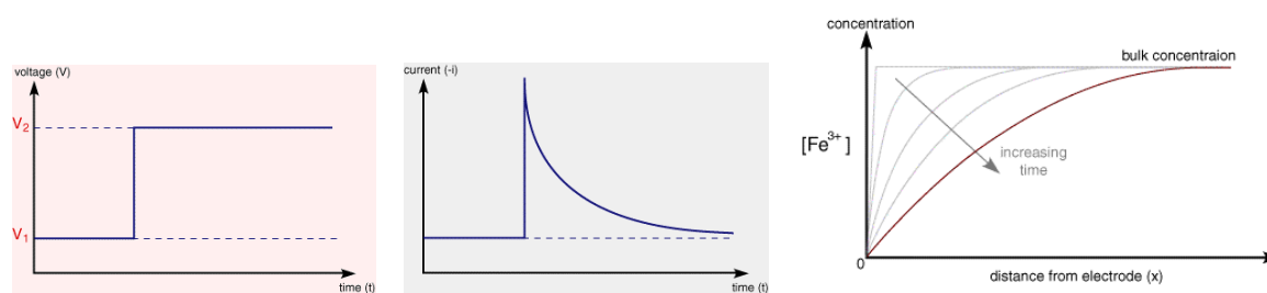
Figure 1.6: Potential step voltammetry: voltage vs time, current versus voltage, and concentration versus distance from the electrode plotted for several times.
