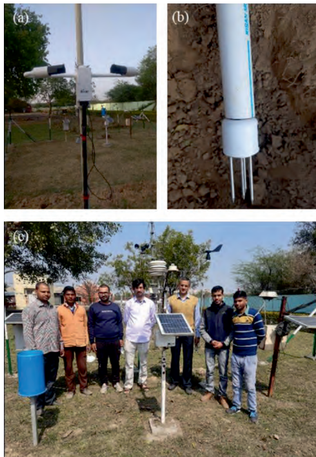
Figure 1. Sensors installed at IIT Kanpur- (a) visibility sensor, (b) soil moisture sensor and (c) automatic weather station.
