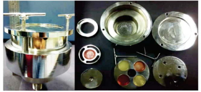
Figure 2 Air Sampling Device and its internal components
