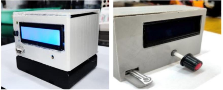
IITK-developed “Portable Readout Unit for Chemiresistive Sensor (PRuCSor)” by Dr. Santosh Kumar Misra and team (IPA No. 202411100478) is available for licensing. This compact, 180g, battery-powered device uses paper-based carbon electrode chips to measure resistance in liquids and features a screen and Bluetooth for easy, portable use.
