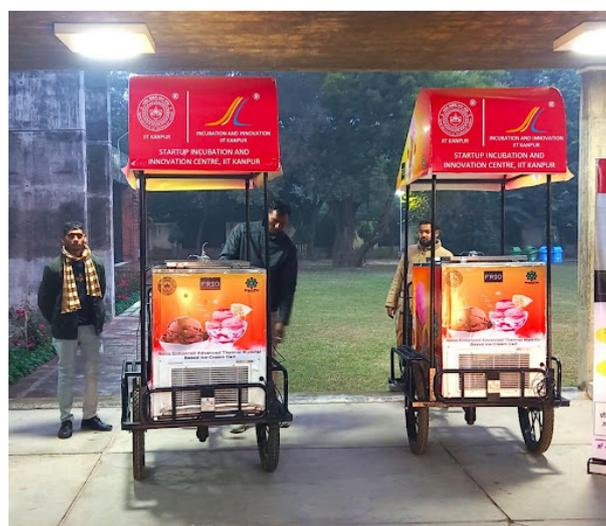
IIT Kanpur has launched a **Phase Change Material-Based Thermal Management System**, developed by Prof. Sri Sivakumar, with the ability to maintain a consistent temperature range (typically  $-20^{\circ}\text{C}$  to  $-10^{\circ}\text{C}$ ).
