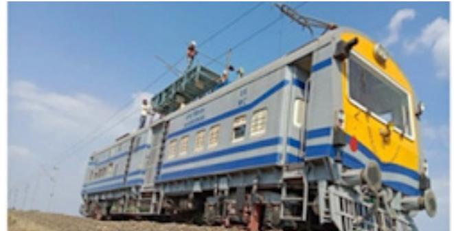
IITK-developed technology, “Fuel Cell and Battery Hybrid Powered Electric Tower Car with DC Traction Motor” (IPA No. 202411068288), by Dr. Prabodh Bajpai, Dr. Amarendra Edpuganti & team, is available for licensing. It replaces diesel-powered tower cars with a zero-emission, fuel-free alternative, combining fuel cells and lithium-ion batteries for efficient, low-maintenance, and sustainable operation.
