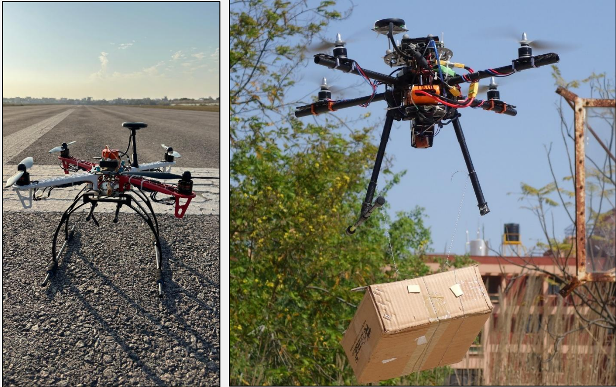
(Left) A GPS-Enabled UAV and (Right) a Heavy-Lift UAV, both designed by Team AR, IITK. These models allowed us to conduct trials for pick-up and delivery services.
