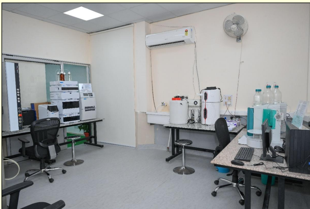
The facilities include an HPLC-GPC system equipped with advanced detection technologies like Evaporative Light Scattering Detection (ELSD), Light Scattering Detectors, UV-VIS and Refractive Index (RI) Detectors
