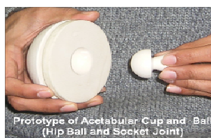
Figure 1: Prototype of Hip Ball and socket joint, which will be replaced by UHMWPE-HA- \text{Al}_2\text{O}_3 -CNT biocomposite after animal studies and clinical trials.
