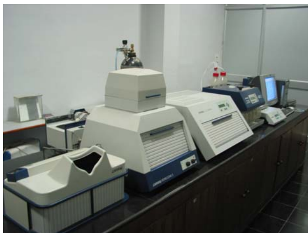
From L to R (front row): Viewing Box, Reprostar, TLC Scanner, AMD2, Linomat 5, Computer with winCATS, plate heater. (Rear) Printer, Plate Coater
