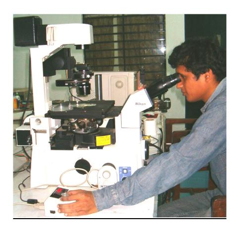
Nikon Eclipse TE2000U is an advanced inverted microscope used for variety of applications which require high precision e.g. live cell microscopy, flow visualization within microfluidic channels, for characterizing interfaces in the area of contact mechanics and so on and so forth.
