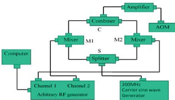
Figure 2. Schematic of the RF mixer to generate desired modulation in the carrier RF frequency.
