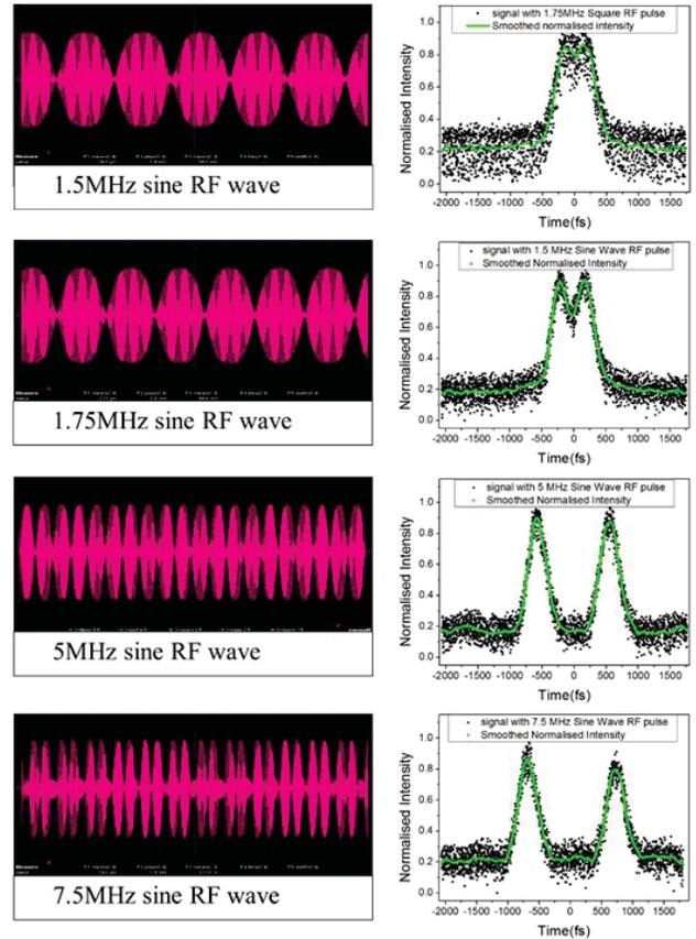
Figure 4. Application of RF sine pulses at certain frequencies from both channel modulation to the AOM (left side) and the corresponding output pulse (right side) as measured through cross-correlation with the original unmodulated pulse. Note the pulse splitting effect.
