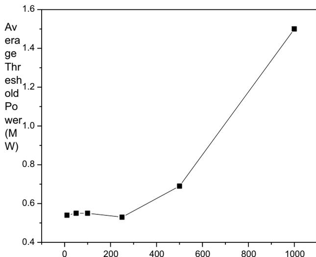
Figure 5. Threshold power needed to generate super-continuum at different repetition rate changes with different laser repetition rate
