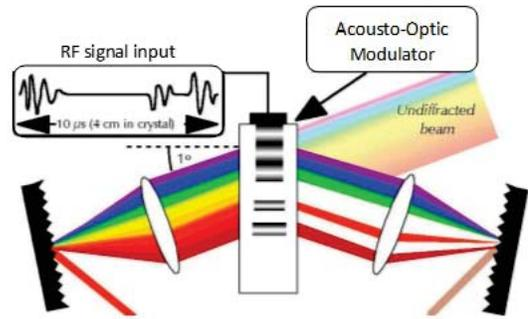
Figure 1. Pulse Shaping schematic: Principle of (a) time domain shaping and (b) frequency domain shaping, which is the more practical one for ultrafast lasers and is translated into (c) Experimental Fourier Optical domain shaping with AOM.
