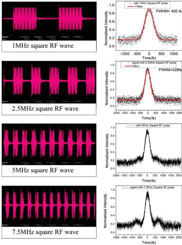
Figure 3. Application of RF square pulses at certain frequencies from only one channel modulation to the AOM (left side) and the corresponding output pulse (right side) as measured through cross-correlation with the original unmodulated pulse.
