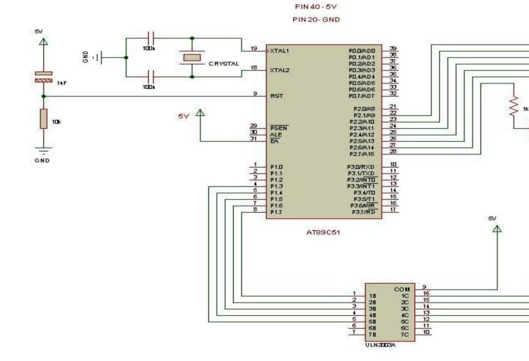
The transistors are turned on by the TTL voltages applied by the Port 2 of MCU to their bases through 1-kilo ohm resistors. To make any led segment glow just make the respective row and column bits on. We send the hex value of character to be displayed in first column to Port2 and send columns selection byte to Port1. Then we send another hex value to row and select the respective column. This process is done very fast and it seems that the whole character is displayed at the same time.
