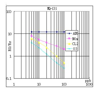
Figure shows the typical sensitivity characteristics of the MQ-131 for several gases. in their: Temp:  $20^{\circ}\,$
