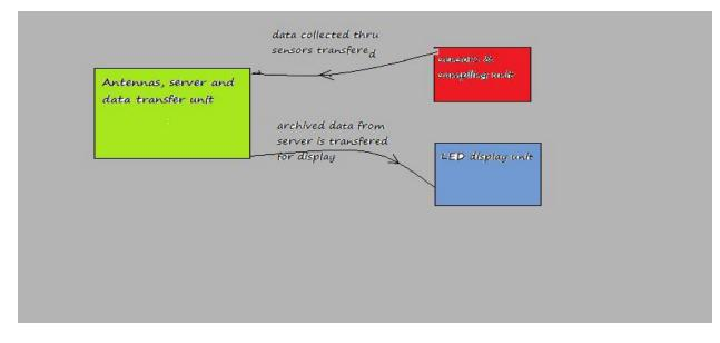
2. Data retrieved from sensor unit will be transferred to the main server through gsm or transreceiver.
