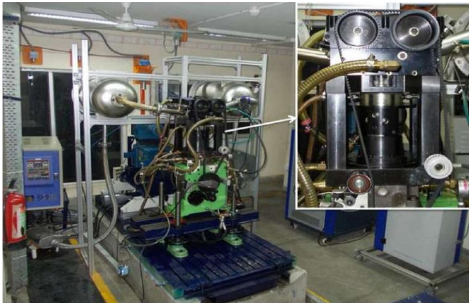
Fig 2: Experimental Setup of GDI Engine with optical head
