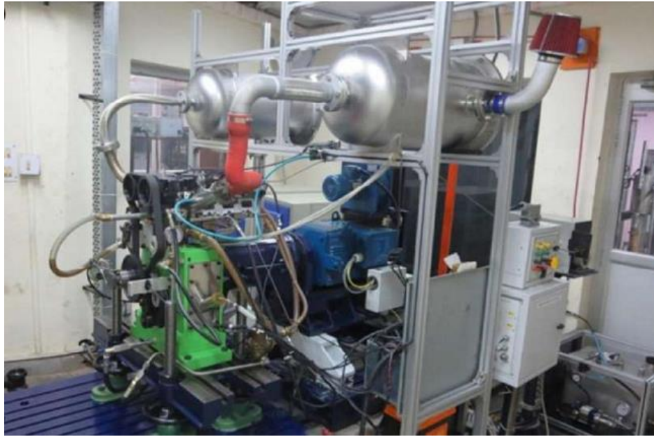
Fig 1: Experimental Setup of GDI Engine with thermal head
