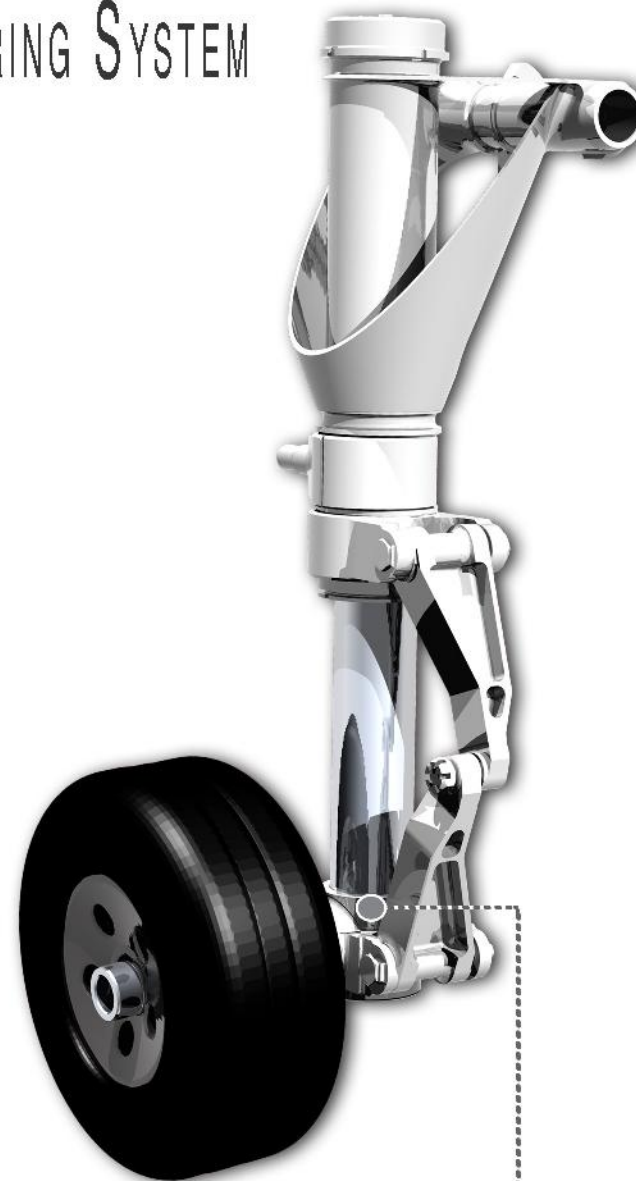
'CAD MODEL OF DORNIER DO-228 AIRCRAFT LANDING GEAR' DEVELOPED FOR UNDERSTANDING THE DESIGN AND ALSO FOR USING IN VARIOUS SIMULATIONS.
