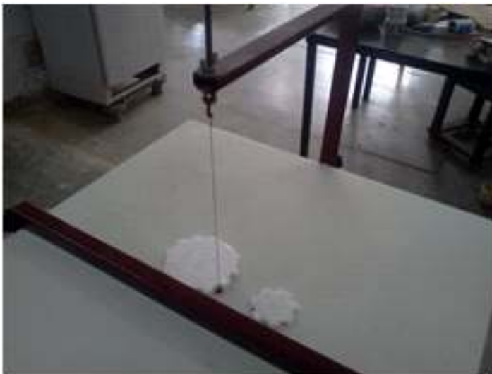
Thermocol cutting machine for shaping very soft grained thermocol.
