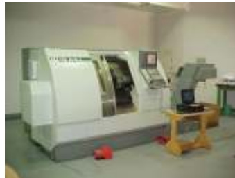
CTX GILDMEISTER TURNING CENTER Spindle Speed 4,500 rpm Controls Fanuc 21i T Turning length-600mm, Dia-305mm
