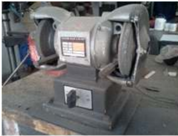
Grinding machine A two grain grinder for polishing cast iron moulds and other Chamfering wood and MDF jobs
