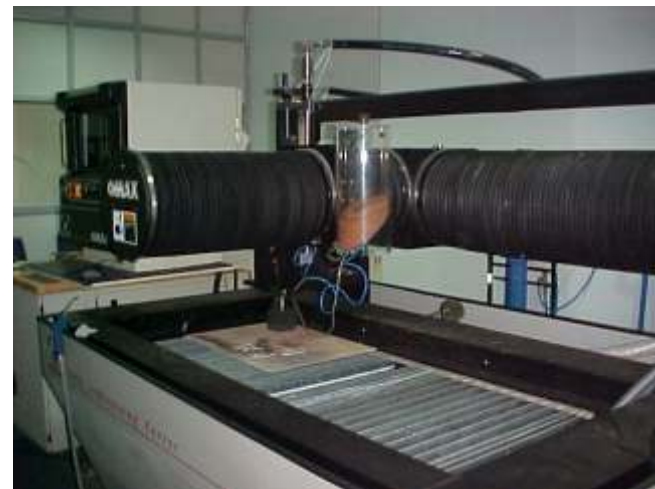
Model OMAX 2652 (above) Speed: 200 in/min; X-Y Travel: 52" x 26" Accuracy: 0.051 mm per 1' travel
