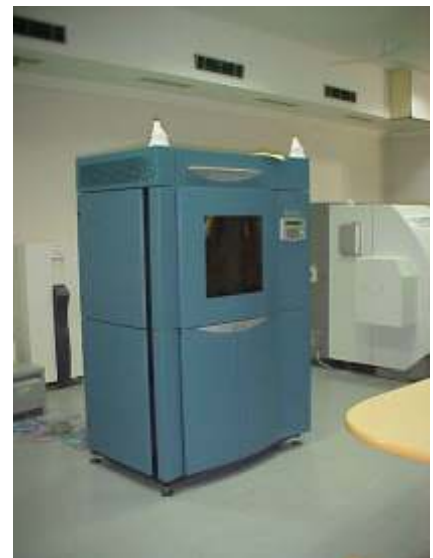
Layer Thickness: 0.005 inch(0.125 mm) Build Size: 16 x 14 x 16 inches (406 x 355 x 406 mm)
