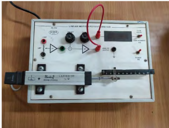
(b) Measurement of linear displacement by potentiometer
