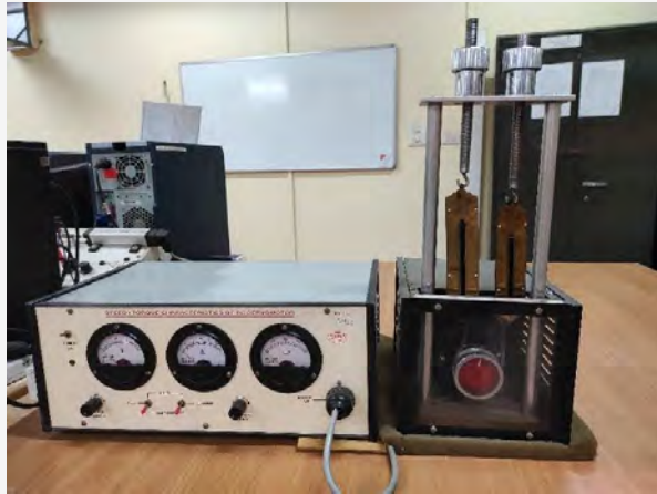
(a) Speed torque characteristics of DC servomotor
