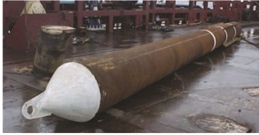
FIGURE 1. A typical deep-penetrating anchor. Typical dimensions are \sim 15 m in length and \sim 1 m in diameter, with a weight of \sim 1 ton. Taken with permission from Interdoor.
