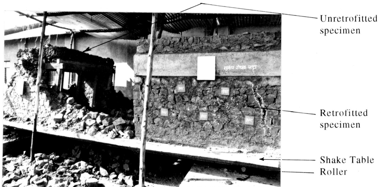
Fig.7 Half scale model rooms tested on shake table (Arya, 1995)
