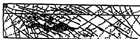
(a) B22 Shear Failure (Slippage at the concrete joint)
