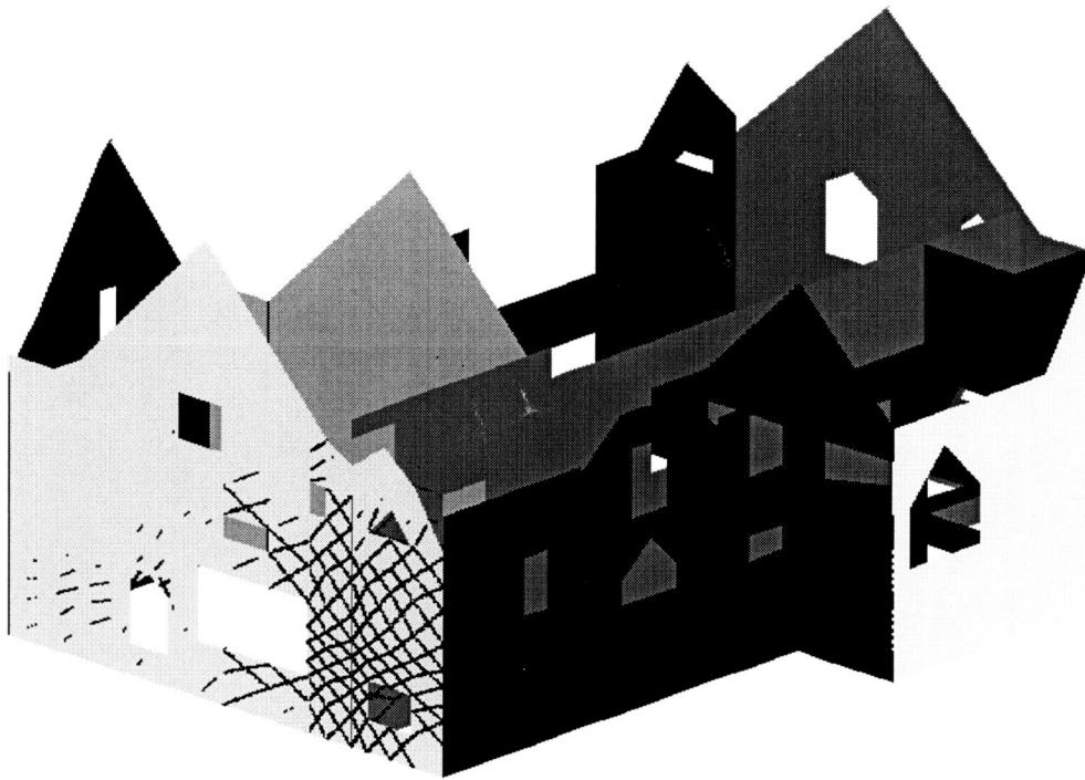
Fig. 6. ANSR-II Model Showing Cracking Rendered in AutoCad
