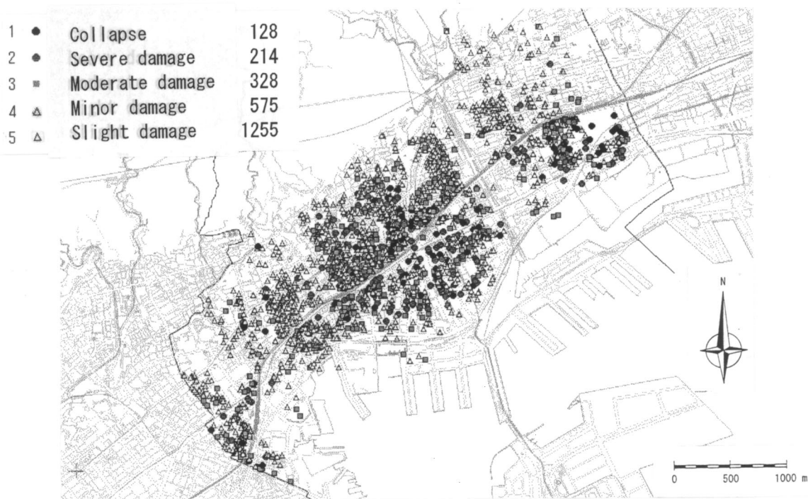
Fig. 4 Distribution of damaged buildings in Chuo Ward, Kobe City.
