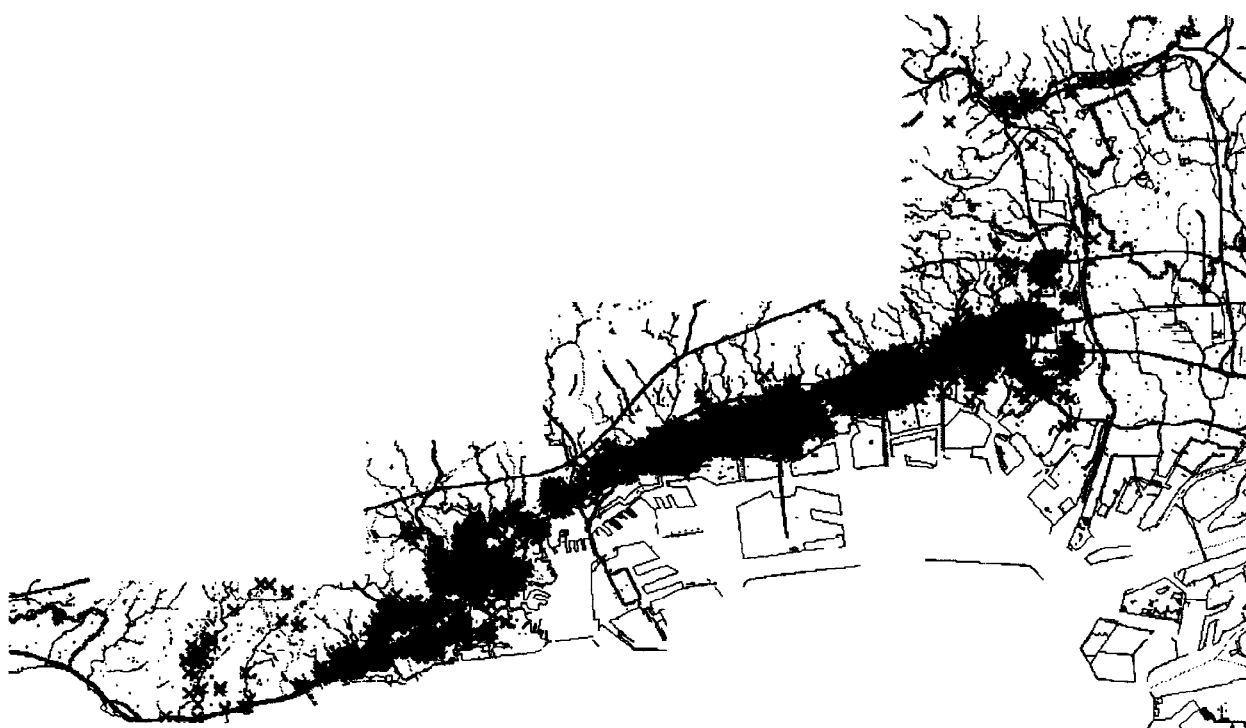
Fig. 3 Distribution of collapsed buildings based on aerial photographs taken by the Geographical Survey Institute (GSI) on January 17 and 20, 1995.
