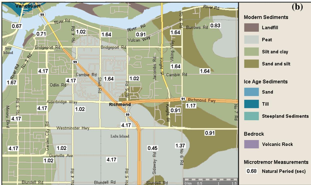
**Figure 4. Site periods obtained from microtremor measurements overlaid on surface geology on: (a) Vancouver side (b) Richmond side of the Fraser River**
