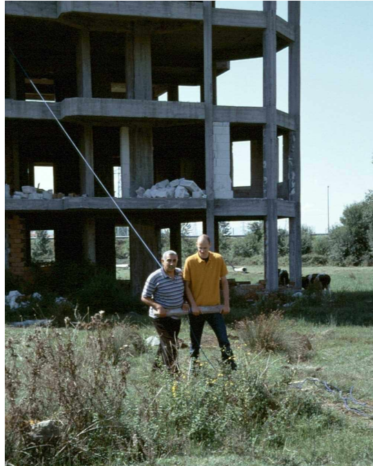
Figure 3. External excitation of the building from the outside produced by manpower.
