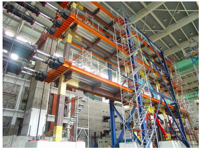
Fig. 1 (a) Plan and elevation of the full-scale CFT/BRB composite frame (b) Photo of the CFT/BRB test frame
