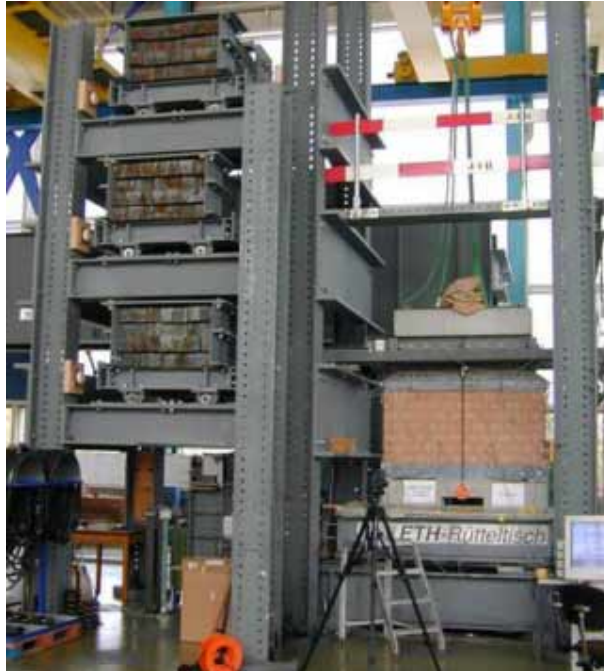
Figure 8: Retrofitted specimen ready to test in the dynamic part
