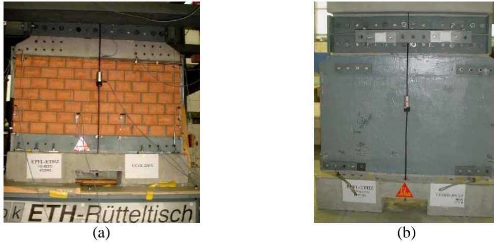
Figure 10: Specimens (a) S1-REFE and (b) S1-WRAP-G-F at the test end of the dynamic tests
