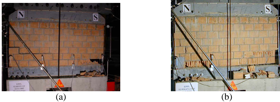
Figure 11: Specimens (a) S2-REFE-ST and (b) S2-WRAP-G-F-ST (unreinforced face) at the test end of the static cyclic tests
