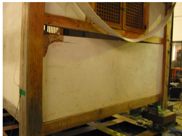
(b) Separation of wall panel from frame at 0.24g
