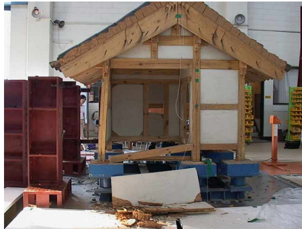
Figure 8. Collapse of wall panel of half-scale model at 0.36g
