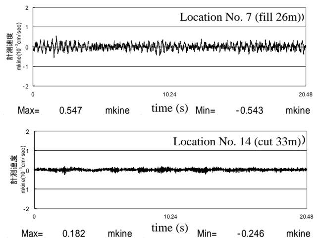
Fig. 4 Samples of velocity wave
