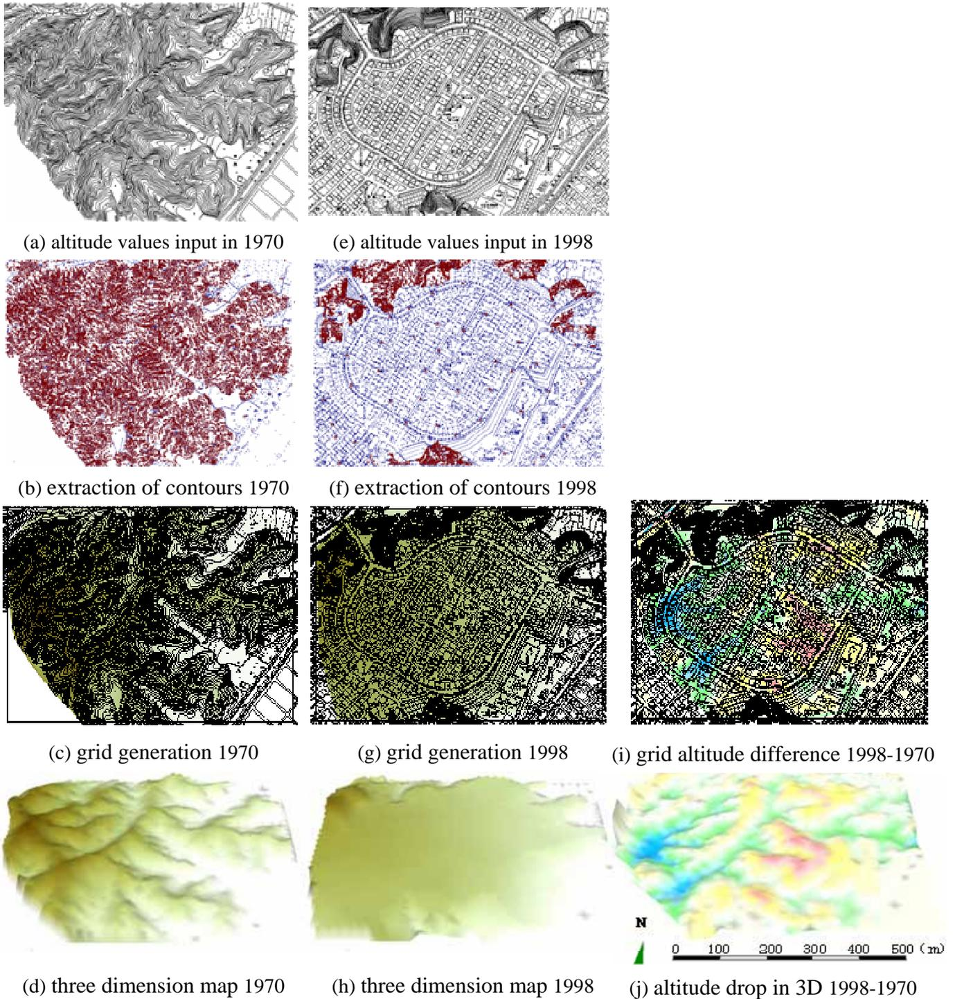
Fig. 1 Making procedure to classify cut and fill ground
