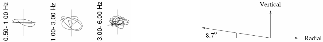
Figure 10: Particle orbits on a vertical plane calculated from borehole accelerograms at the onset of S-wave portion of the main shock. The orbits are calculated from band-pass filtered waves in the frequency range of interest.
