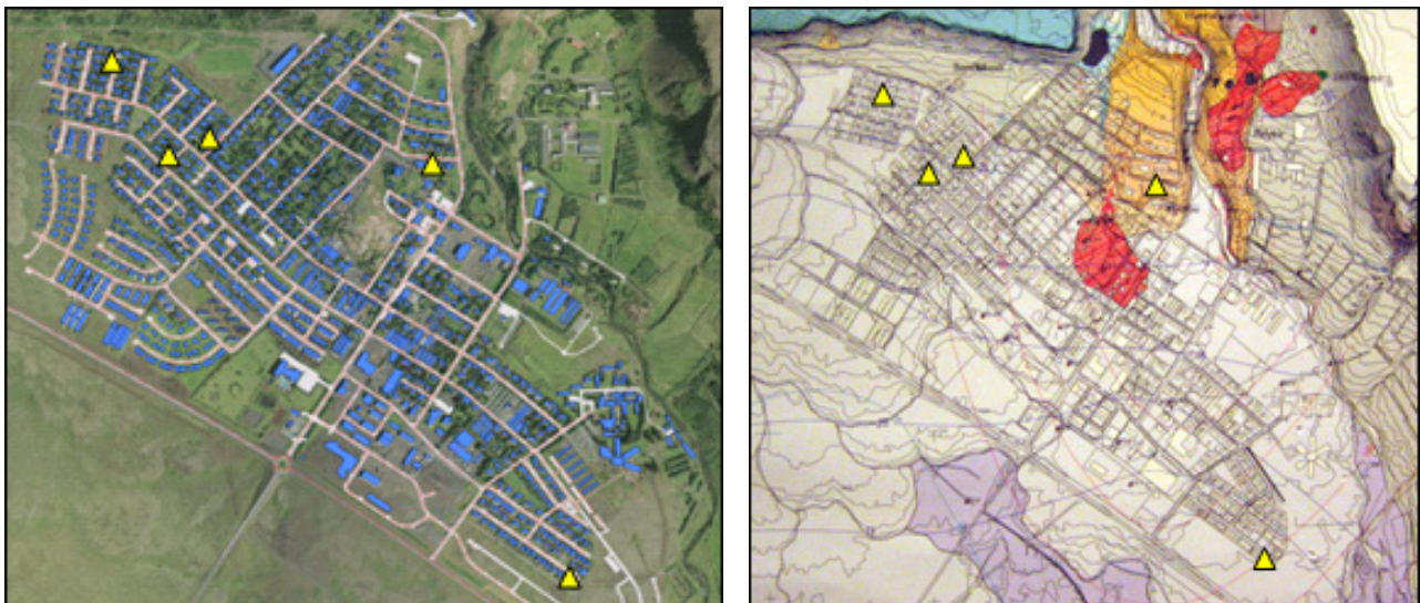
Figure 2 The street-and-structural layout (left) of the town of Hveragerdi where the pre-field study was carried out. The triangles denote the station locations of the test-setup, located in residential structures. A schematic map showing main geological features of the town area (right) shows that the town resides largely on a single lave field. The red and orange areas denote high geothermal activity.
