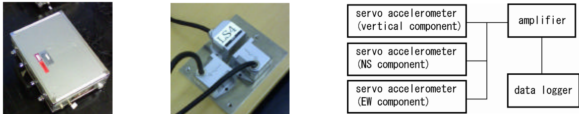
Fig.7 Left: appearance of three component portable seismometer (AKASHI GPL), center: servo accelerometer (RION LS-10C), and right: configuration of the recording system.
