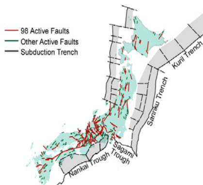
Figure 1. The plot shows the Philippine Sea and Pacific subduction zones segments, eastern Japan Sea convergence front and the active and potentially active crustal faults.
