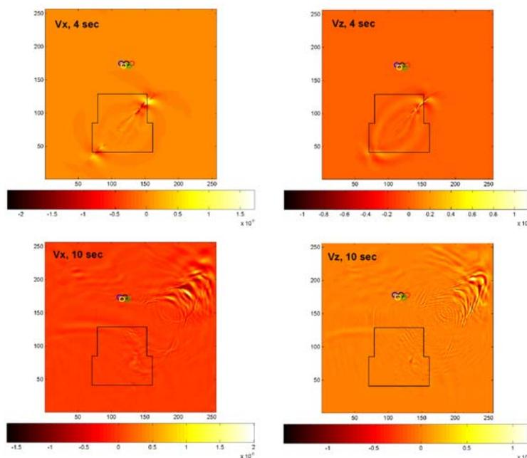
Figure 4. The snapshots of the horizontal and vertical components (Vx, left column and Vz, right column, respectively) of the particle velocity on surface at 4 and 10 seconds after the rupture of a vertical fault.
