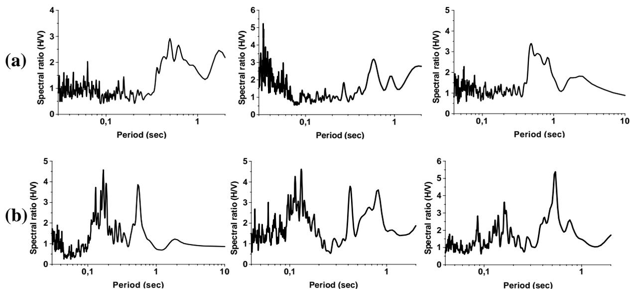
Figure 3. Examples of spectral ratios in Villa de Alvarez town. (a) Sites located in the undamaged zone; (b) Sites located in the heavily damaged zone.
