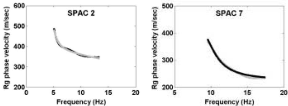
Figure 7. Theoretical phase velocity dispersion curves (grey lines) corresponding with the respective optimum models and measured dispersion curves (black lines).
