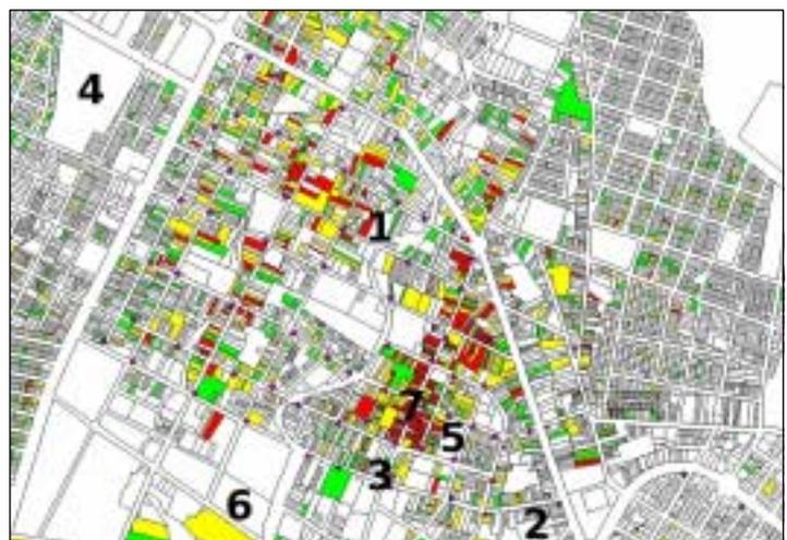
Figure 2. Distribution of damaged buildings in Villa de Alvarez (red block: heavy damage; green block: middle damage; yellow block: slight damage) and location of SPAC sites (Numbers: 1-7)
