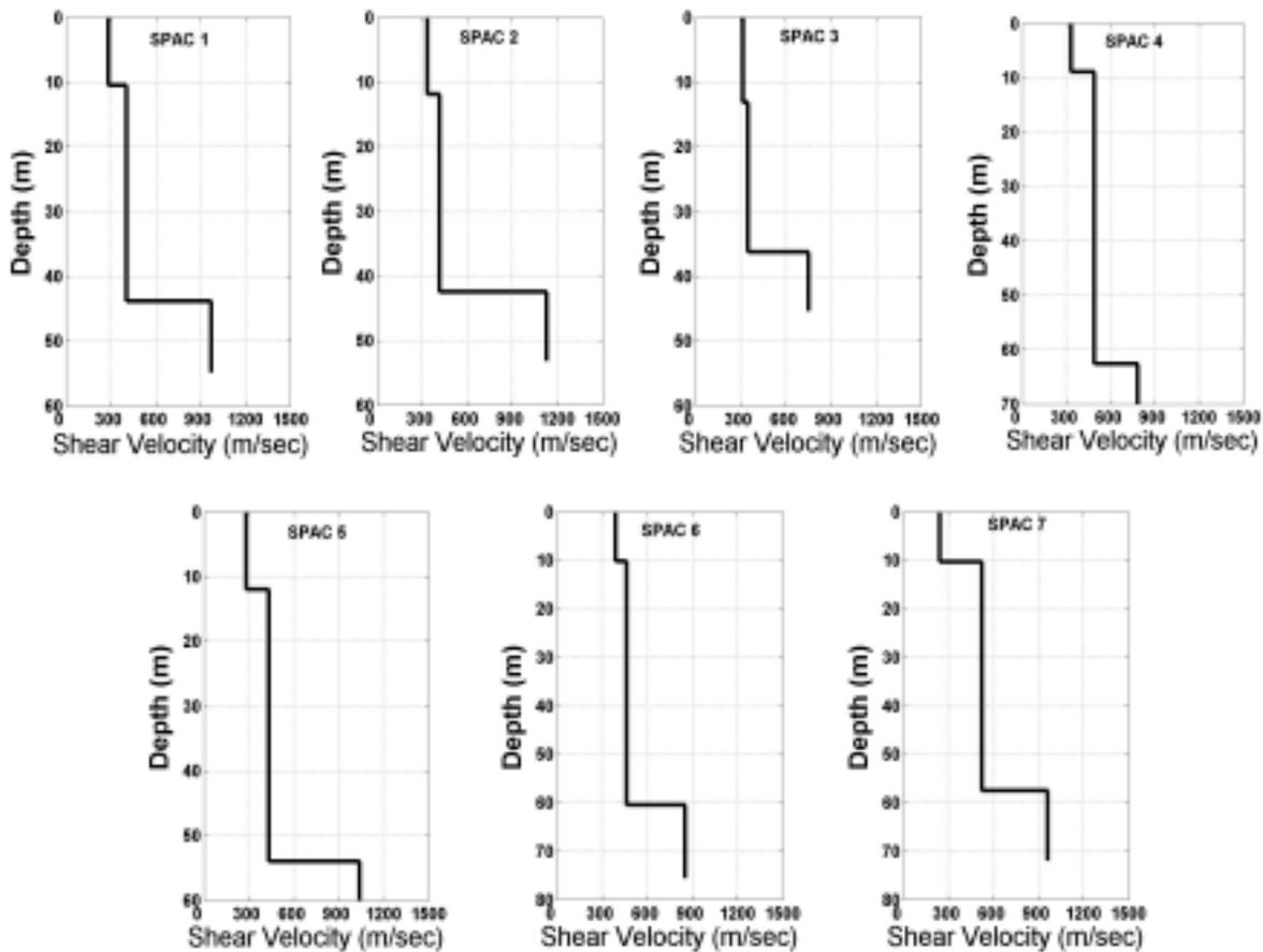
Figure 6. Shear-wave velocity models derived from inversion of phase velocities of Rayleigh waves.
