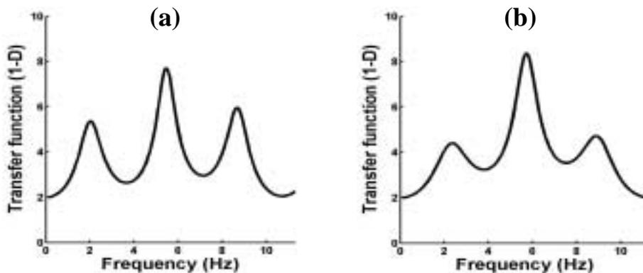
Figure 8. Example of transfer function calculated for some ground models in the damage zone. (a) SPAC 5; (b) SPAC 7.
