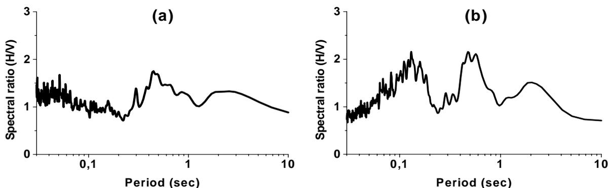
Figure 4. Site effect characteristics from H/V spectra: (a) Undamaged zone; (b) Heavily damaged zone.
