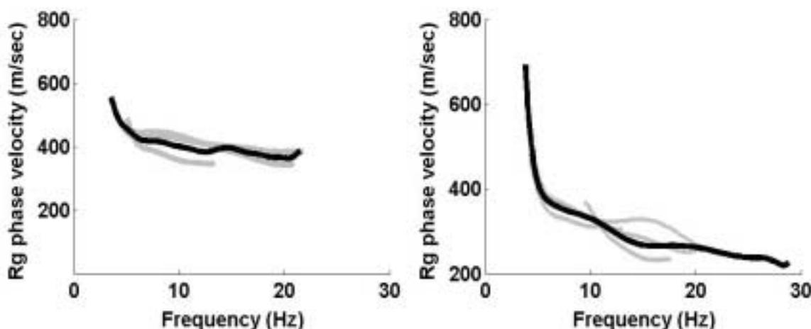
Figure 5. Rg-wave phase velocities (grey lines) measured at the SPAC sites and respective mean velocity curves (black lines). (a) Undamaged zones (SPAC 2, 4, 6). (b) Damaged zones (SPAC 1, 3, 5, 7).
