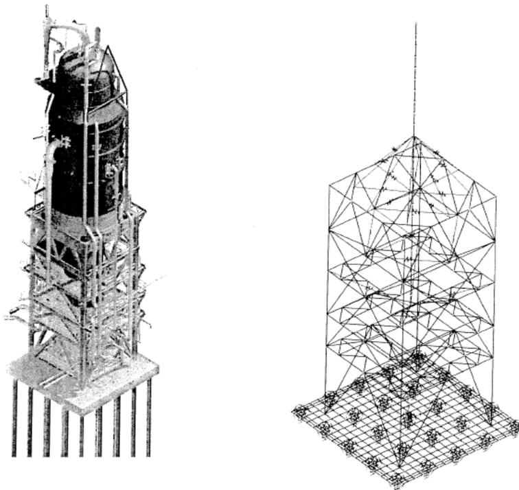
(A) View original model of as-built structure (B) FEM model for seismic analysis
