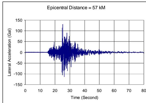
Fig. 2 Horizontal ground acceleration from an earthquake record
