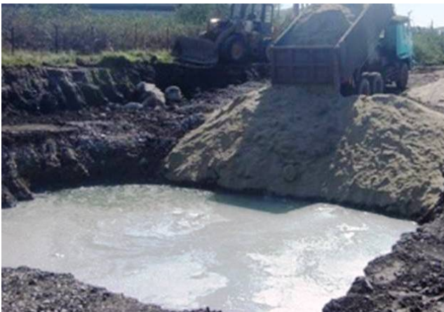
Photo 1 In situ test site (6mW, 8mL, 5mD) filled with Granulated Blast Furnace Slag.
