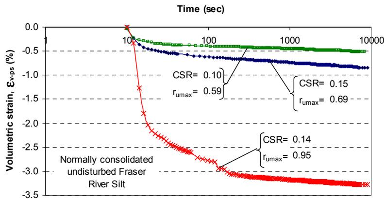
Figure 4. Typical post cyclic volumetric strain following cyclic loading of Fraser River silt.
