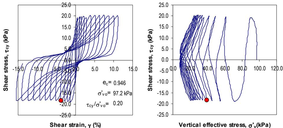
Figure 2. Constant volume cyclic DSS response of Fraser River Silt at CSR = 0.20.
