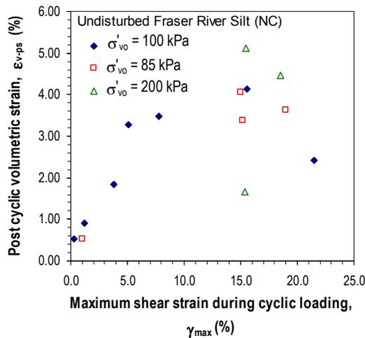
Figure 6. Post-cyclic consolidation settlements versus maximum cyclic shear strain developed during constant volume cyclic DSS loading.
