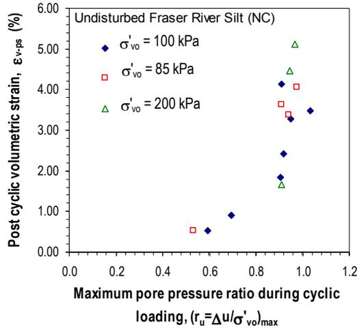
Figure 5. Post-cyclic consolidation settlements versus maximum excess pore water pressure ratio developed during constant volume cyclic DSS loading.
