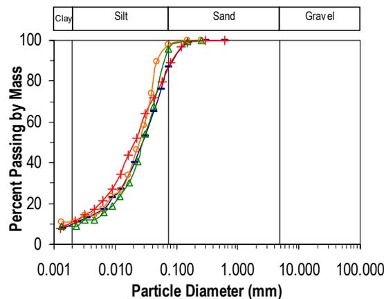
Figure 1. Grain size distribution of natural Fraser River Delta silt
