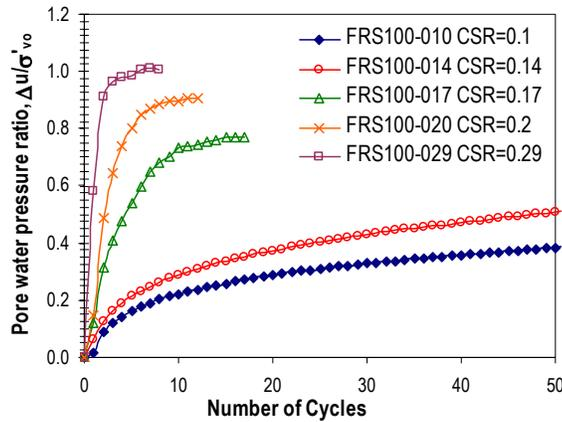
Figure 3. Excess pore water pressure ratio during constant volume cyclic DSS testing of Fraser River silt.
