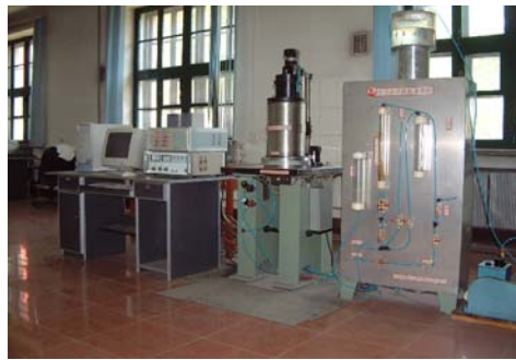
Figure 1 The resonant column device used in tests
