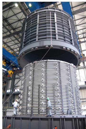
Photo 3 Laminar box being covered for saturation
