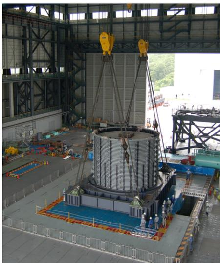
Photo 2 Laminar box carried by two cranes
